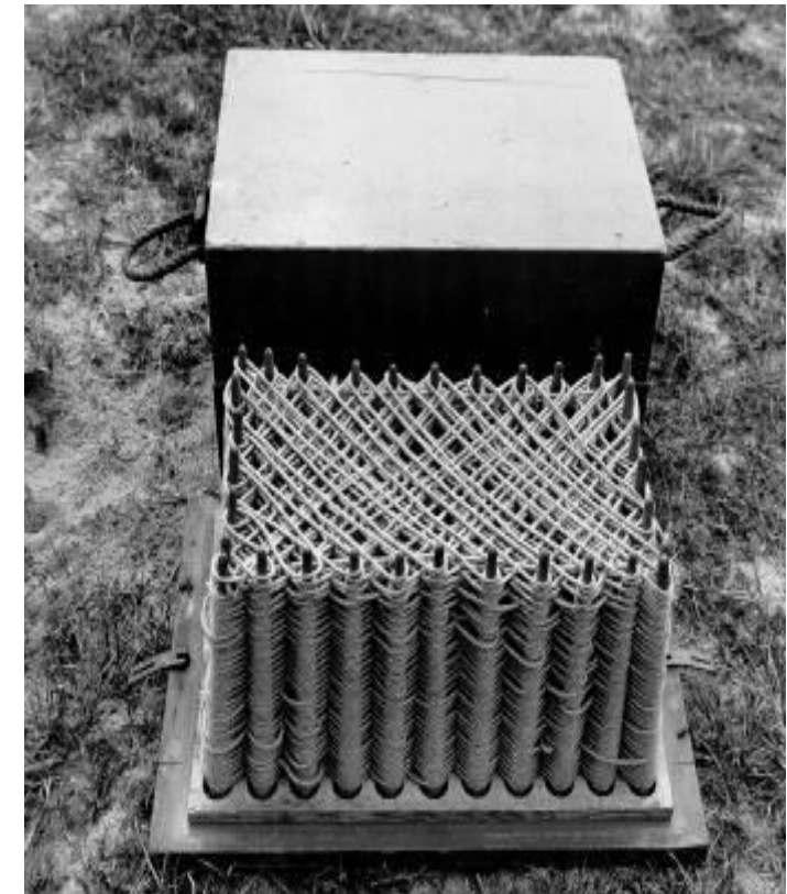
METHOD OF WITHDRAWING FRAME AND PINS FROM SHOT-LINE IN FAKING-BOX.
